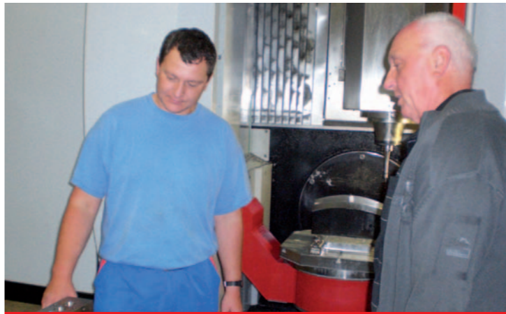
Swivel table. The swivel rotary table is controlled by state-of-the-art torque motors. This technology guarantees highly-precise positioning and interpolation throughout the machine's entire service life. As opposed to worm gears driven axis, it does not cause any wear on the machine. Backlash and positional hysteresis are entirely eliminated. The integrated water cooling system provides a constant temperature, even in highly dynamic applications.
