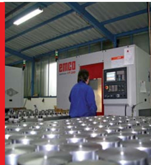
Quick loading through the spindle’s direct pick-up of the raw material
