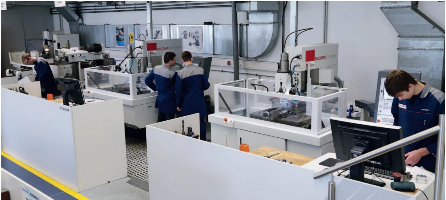
Since September 2016, two new FB-600 MC universal milling machines have been completing Haidlmair's vocational training centre. One machine is equipped with a Siemens 828D control while the other one is operated via a Heidenhain TNC 620.
