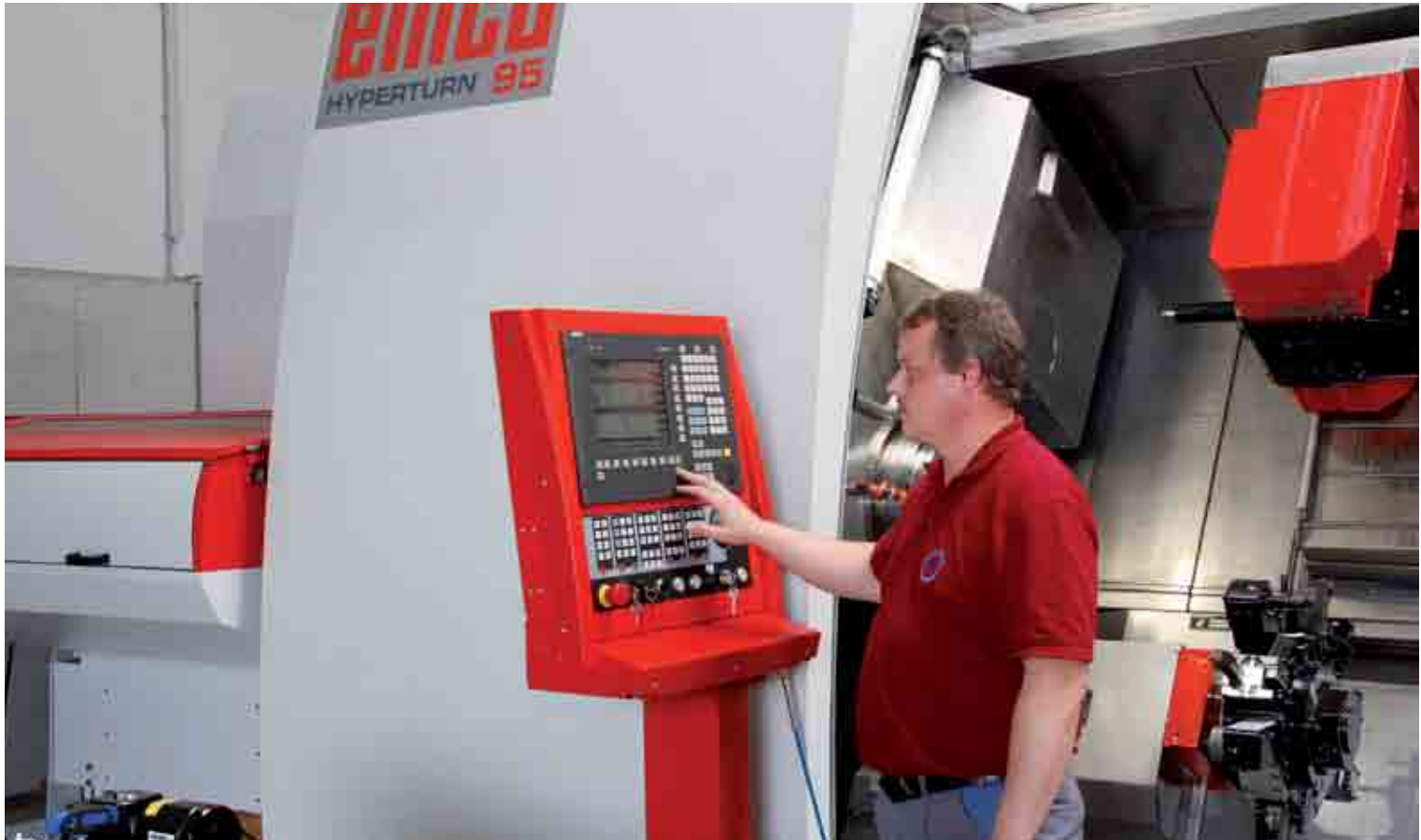
At MKE, programming tasks are performed with the ESPRIT CAM system, and also directly at the machine using the Sinumerik 840D-sl by Siemens. (note: pictured – Andreas Schramel, CNC Machinist)
